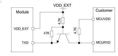
Figure 25: TX level converting by transistor
