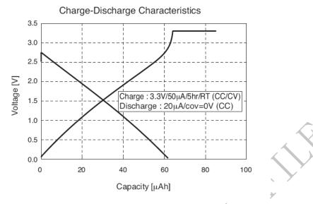
Figure 21: Seiko XH414H-IV01E charge-discharge characteristic
