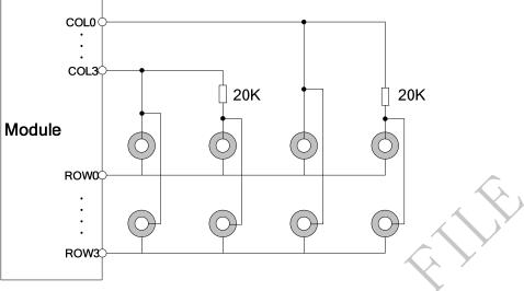
Figure 44: Extended keypad reference circuit
