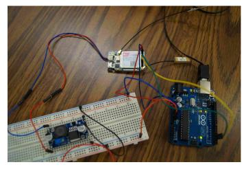
Fig. 8: GSM/GPRS/GPS Working Prototype
