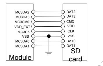
Figure 42: SD reference circuit
