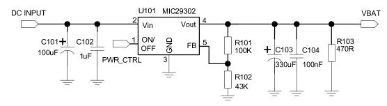
Figure 6: Reference circuit of the LDO power supply
