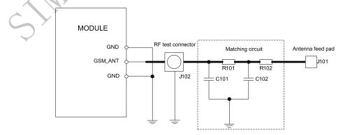
Figure 50: GSM antenna matching circuit
