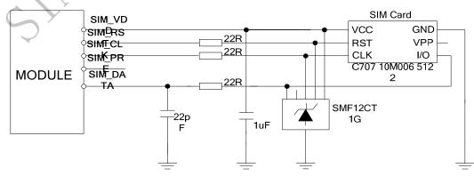
Figure 37: Reference circuit of the 6-pin SIM card holder
