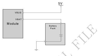
Figure 17: SIM808 with battery charger and pack connection
