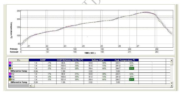
Figure 53: Typical Solder Reflow Profile
