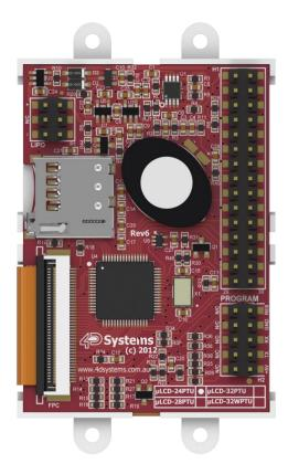
The **uLCD-24PTU** has a **2.4**" TFT LCD display at the forefront of the design that showcases the power and capabilities of the PICASO processor. Combining a resolution of **240x320** pixels with **65K** True to Life colours, this module is perfect for animations, slideshows and other multimedia presentations.
