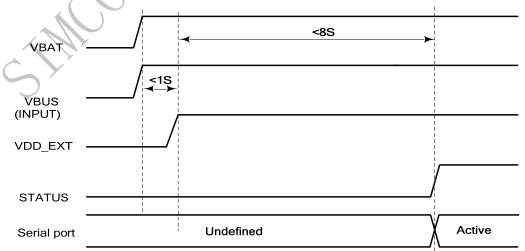
Figure 13: Timing of power on module
