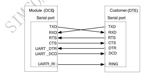
Figure 22: Connection of the serial port
