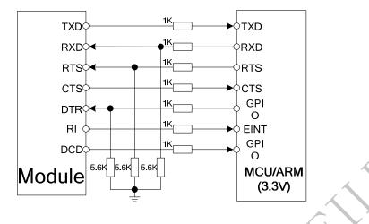
Figure 23: Level converting by resistor
